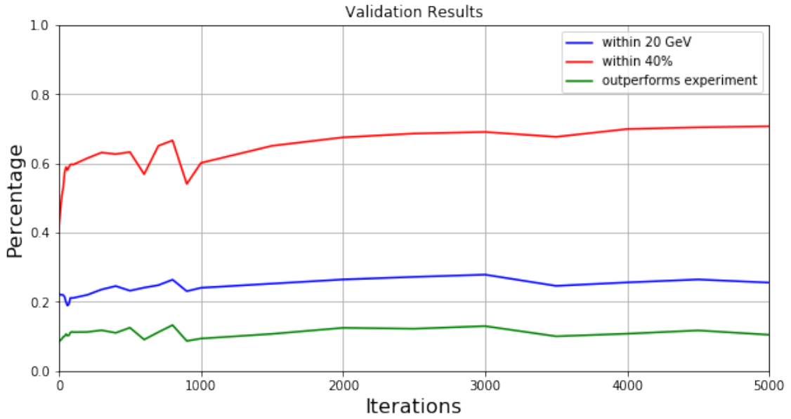
Fig. 3: This figure depicts the performance of the network on the test set as a function of the number of training iterations performed. It uses a number of measures: the percentage of output values within 20 GeV of the true P_T , the percentage within 40% of the true P_T , and the percentage more accurate than standard experimental algorithms.
