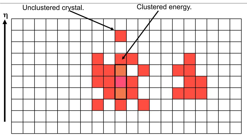
A 1x3 domino about seed cell. If there is sufficient energy, the "wing" cells will be added to make a 1x5
