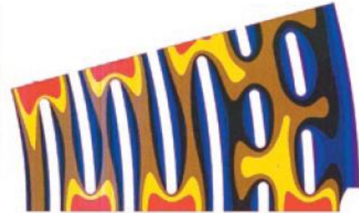
Figure 3. Mid-plane stress of the new A2 coil.
