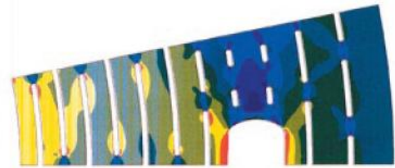
Figure 2. Mid-plane temperature of the new A2 coil.
