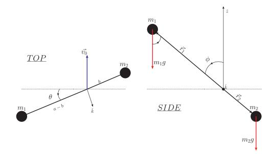
The motion of this system is more easily understood as the superposition of the translational motion of the center of mass (CM) and the rotational motion of the two bobs with respect of to the center of mass.
