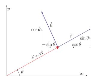
Starting from the position vector for a planar motion in polar coordinates
