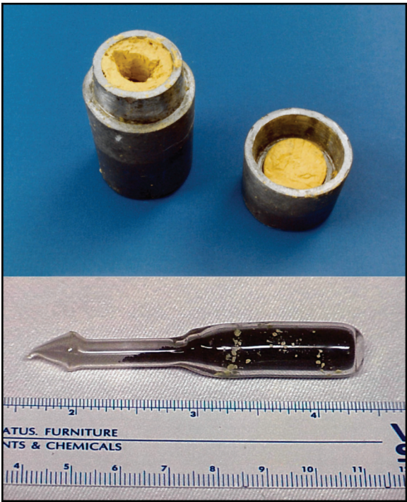
FIGURE FOR 1 Lead container and the glass ampoule containing highly enriched 235 -uranium seized in Bulgaria in 1999 and analyzed at Lawrence Livermore National Laboratory for forensic purposes. SOURCE: “Forensic Analysis of a Smuggled HEU Sample Interdicted in Bulgaria,” UCRL-ID-145216, August 2001.
