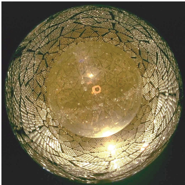
FIGURE 2.35 The SNO detector viewed with a fisheye lens. The central acrylic vessel containing 1,000 tons of heavy water ( D_2O ) is 12 m in diameter and surrounded by 9,500 photomultipliers. SOURCE: Courtesy of SNO.
