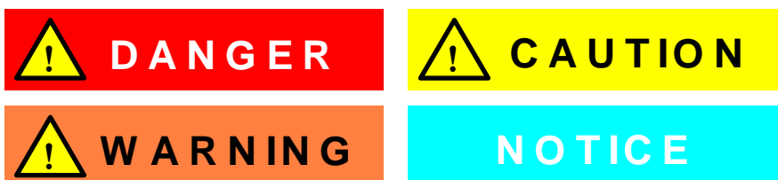
Figure 5.20 Color-coding of safety symbols used to identify dangers, warnings, cautions, and notices in instructions.
