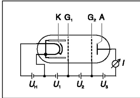
Fig. 2: Franck-Hertz tube (schematic).
