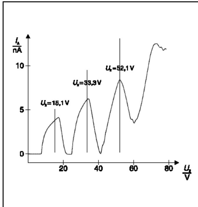
Fig. 6. Franck-Hertz curve for neon (obtained with an XY-recorder)
