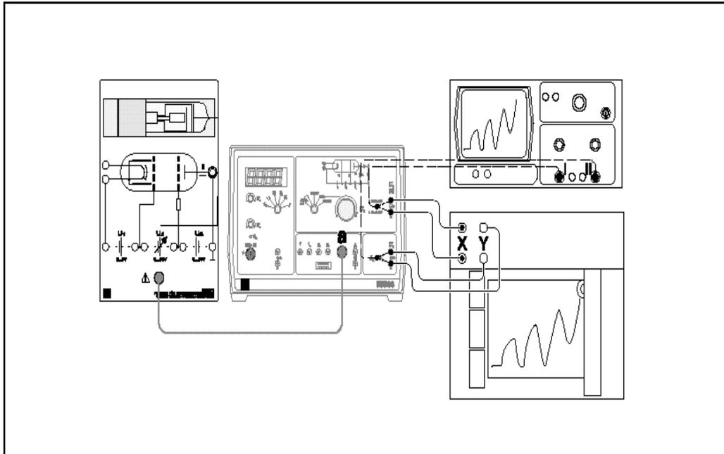
Fig. 4: Experiment setup for Franck-Hertz Neon experiments (don't use the recorder shown).
