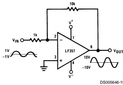
For distortion  $\leq 1\%$  and a 20 Vp-p  $V_{OUT}$  swing, power bandwidth is: 500 kHz.
