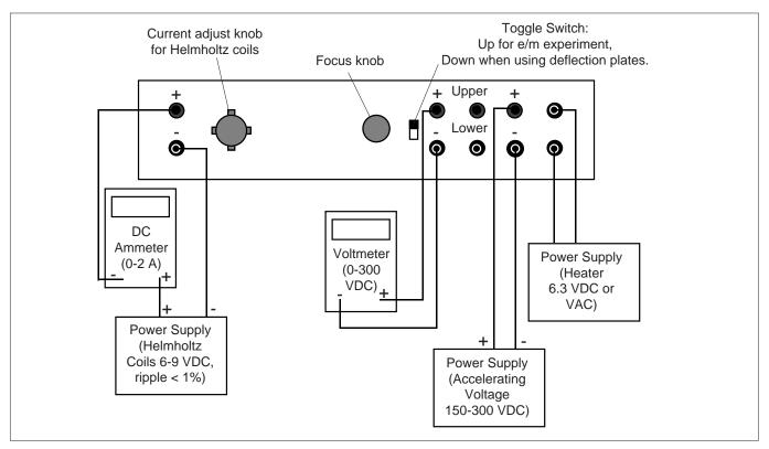
Figure 4 Connections for e/m Experiment
