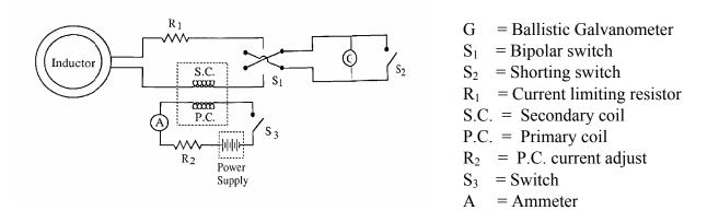
The bottom circuit (one with S<sub>3</sub> and power supply) is a calibration circuit.
