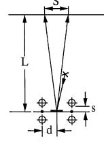
The torsion constant D can be derived from the period of torsional oscillation T of the torsion pendulum:
