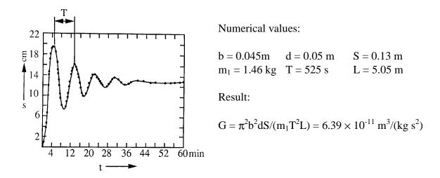
4.7. The value determined is subject to the following *systematic error*: The small sphere will also be attracted by the more distant second large sphere with a very much smaller force F'<sub>o</sub> (see Fig. 3)
