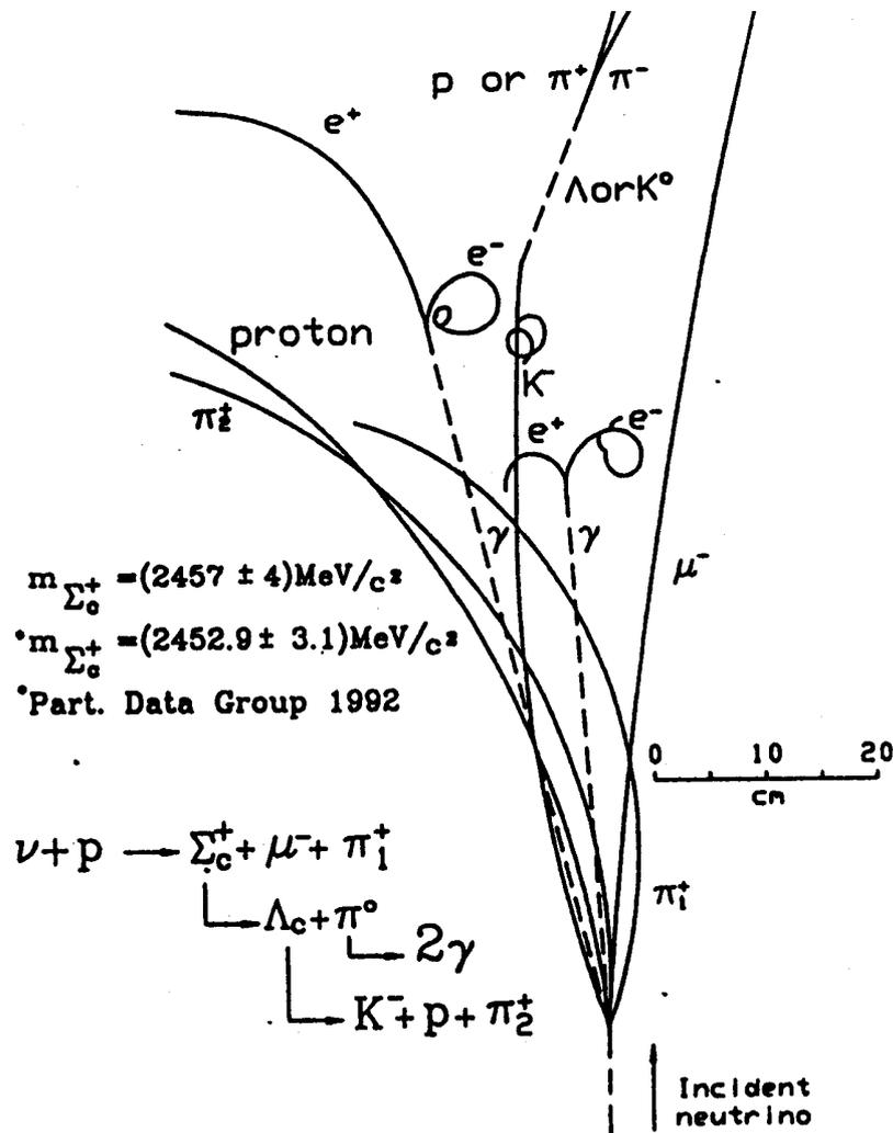
Figure 8: First observation of the production and decay of a completely reconstructed  $\Sigma_c^+$ .
