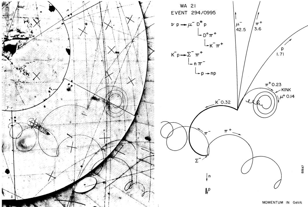
Figure 6: The production of a  $D^*$  charmed particle by a neutrino in BEBC filled with hydrogen.
