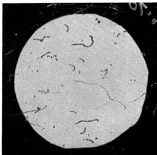
FIG. 2. Photograph of the two-inch ether chamber taken 6.7 milliseconds after the expansion began. The operating conditions were the same as in Fig. 1 except that the radium source was eight inches from the chamber center in the plane of the photograph. Since the chamber had been sensitive for 1.7 milliseconds when this picture was taken, there are a number of "old" electron tracks characterized by larger bubbles than mark the "recent" tracks.
