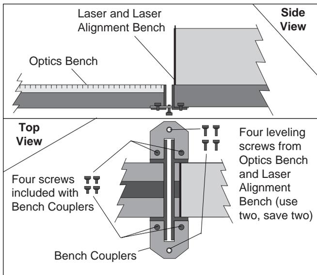
**Figure 7:** Coupling the Optics Bench and the
