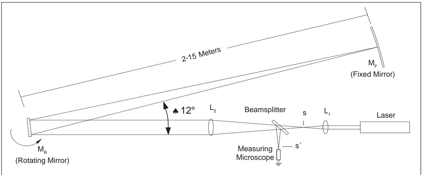
**Figure 11: Positioning the Fixed Mirror ( $M_F$ )**
