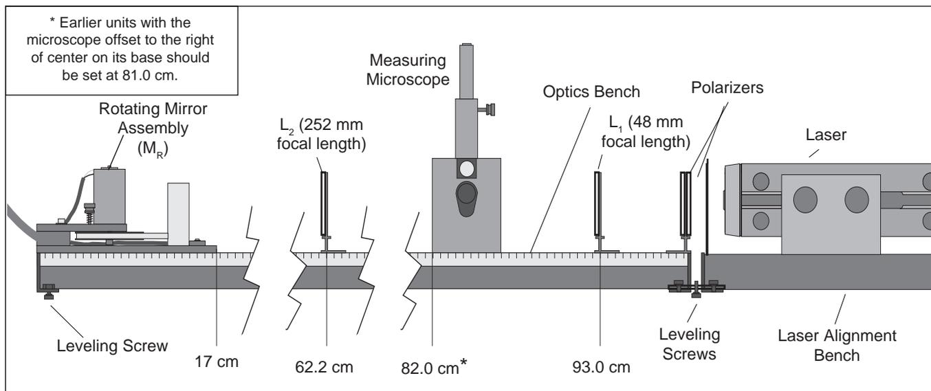
**Figure 5:** Equipment Alignment
