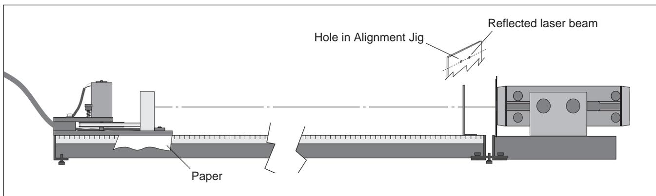
**Figure 9: Aligning the Rotating Mirror ( $M_R$ )**
