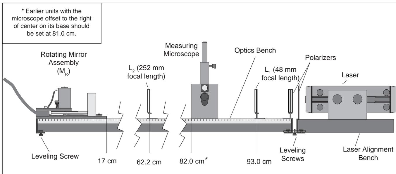
Figure 14: Equipment Alignment
