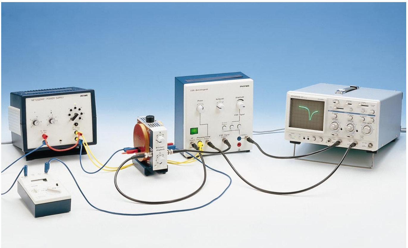
Fig. 1: Experimental set-up for determining characteristic curves.
