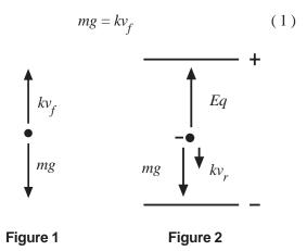
Figure 2 shows the forces acting on the drop when it is rising under the influence of an electric field. In Figure 2, E is the electric intensity, q is the charge carried by the drop, and  $v_r$  is the velocity of rise. Adding the forces vectorially yields:
