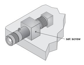
Figure 12. Location of viewing scope set screw
