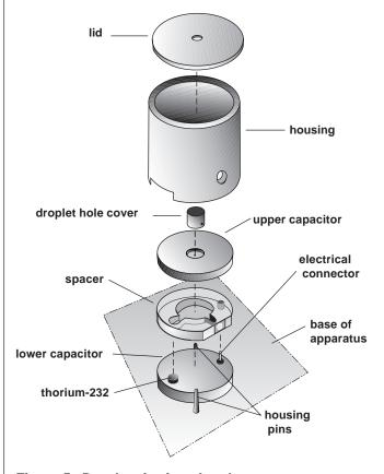
Figure 5. Droplet viewing chamber
