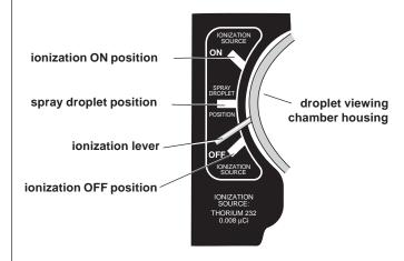
Figure 8. Ionization source lever settings
