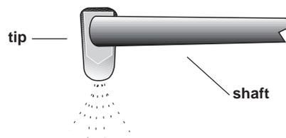
**Figure 9. Correct position of the atomizer tip**
