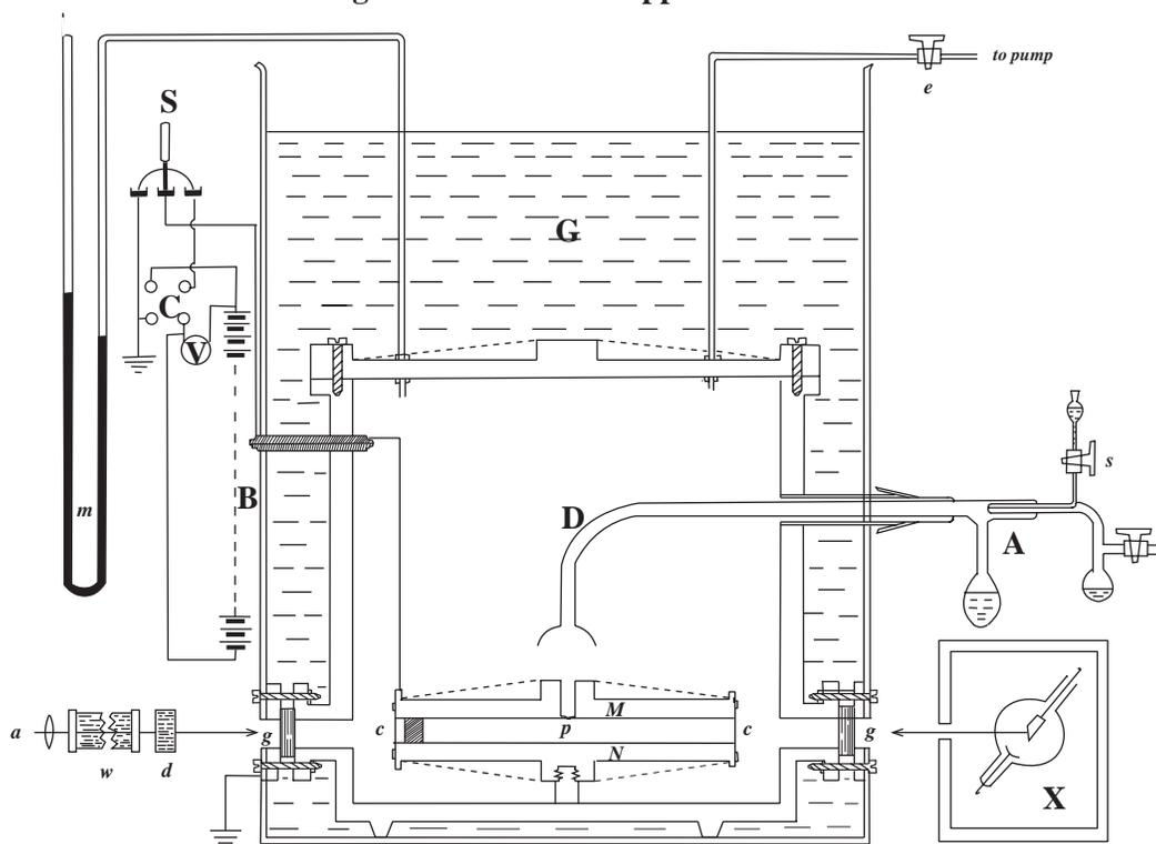
Fig. 11.—A, atomizer through which the oil spray is blown into the cylindrical vessel D. G, oil tank to keep the temperature constant. M and N, circular brass plates, electrical field produced by throwing on 10,000-volt battery B. Light from arc lamp a after heat rays are removed by passage through w and d, enters chamber through glass window g and illuminates droplet, p between plates M and N through the pinhole in M. Additional ions are produced about p by X-rays from the bulb X.
