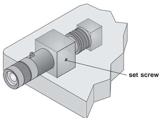
**Figure 12.** Location of viewing scope set screw
