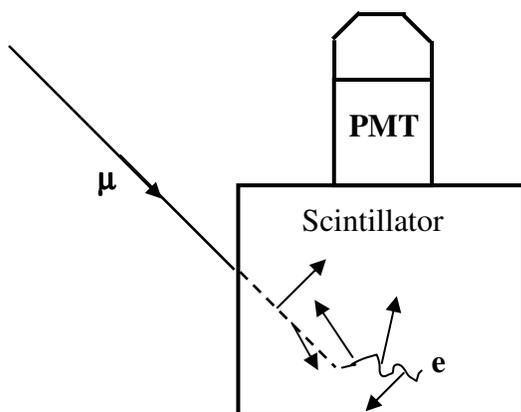
**Figure 2.** Schematic showing the generation of the two light pulses (short arrows) used in determining the muon lifetime. One light pulse is from the slowing muon (dotted line) and the other is from its decay into an electron or positron (wavy line).
