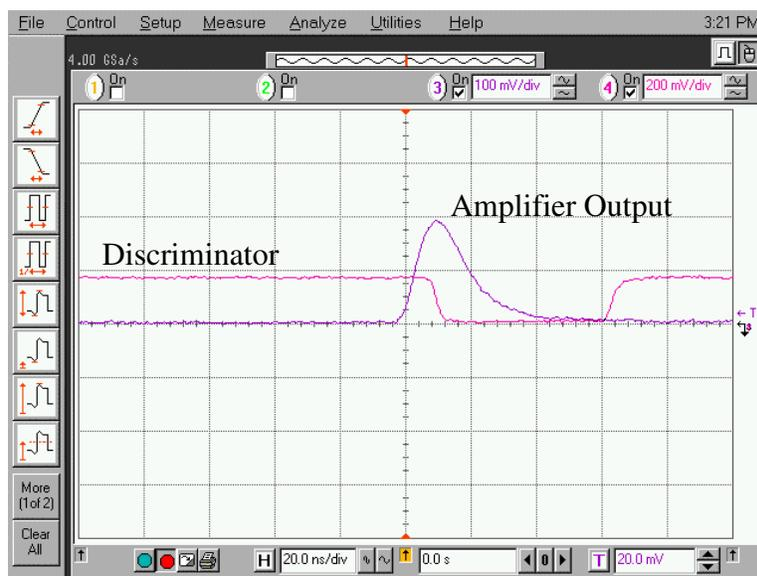
**Figure 10.** Amplifier output pulse from the input signal from figure 9 and the resulting discriminator output pulse. Horizontal scale is 20 ns/div and the vertical scale is 100 mV/div (amplifier output) and 200 mV/div (discriminator output).
